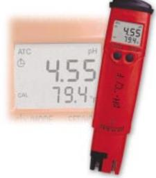
The pHep<sup>®</sup>'s replaceable electrode has a pull-out cloth junction. When the cloth junction becomes dirty from routine testing, simply pull out 3 mm (1/8") to rejuvenate the electrode.
